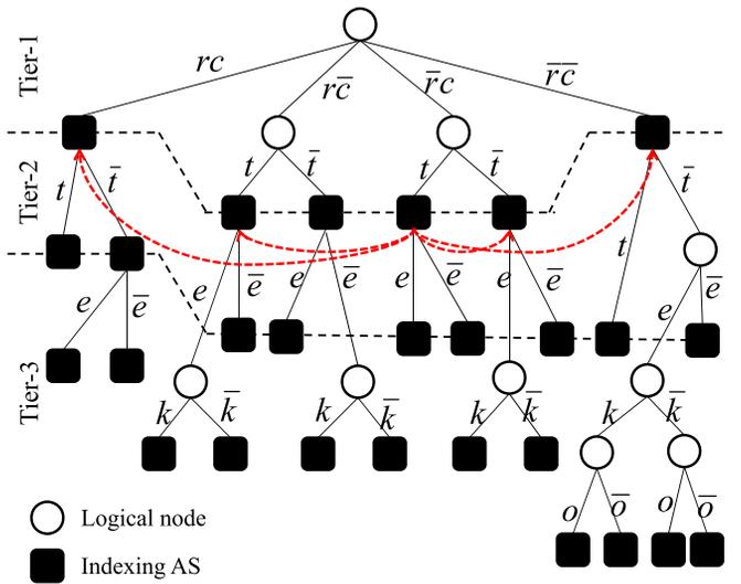
Fig. 2. Mapping a partitioning tree to AS-topology.
